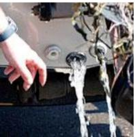
**2. DRAIN** water-related equipment (boat, ballast tanks, portable bait containers, motor) *and* drain bilge, livewell and baitwell by removing drain plugs before leaving a water access or shoreline property. **Keep drain plugs out** and water-draining devices open while transporting watercraft.
